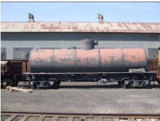
Steel Tank Car Truck Showing Poling Pocket
