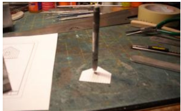
Photo # 5 A pin pushed in at the corners of the doors and windows assists the material from cracking and cuts running too far.
