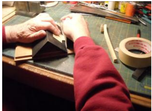
Photo #4 Sanding 45-degree angle on the matching corners.
