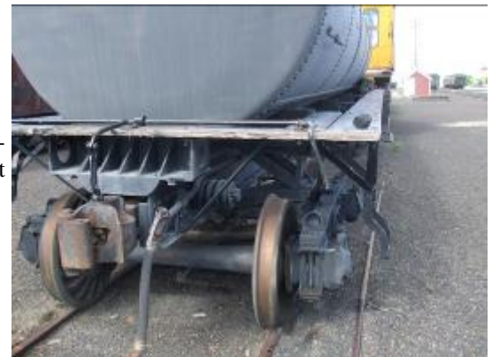
Steel Tank Car Truck Showing Poling Pocket
