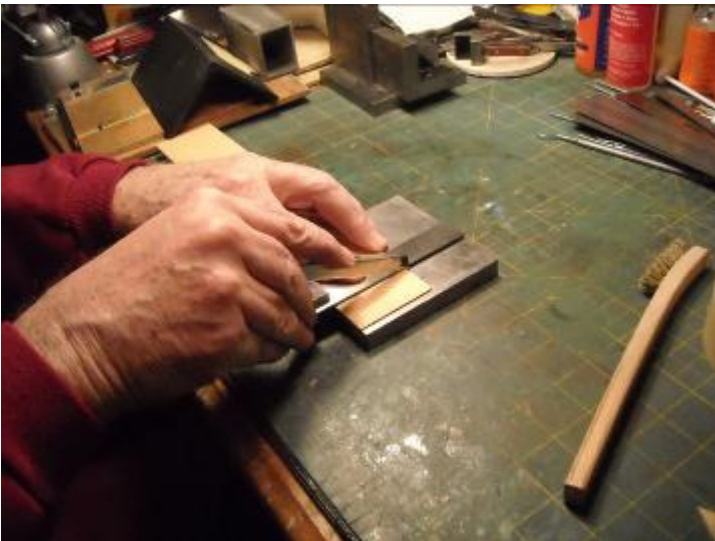
Photo # 1 Note that I always use a faceplate (the flat steel plate machined to be flat and square) and a machinist square to ensure the parts end up correct. I am using an Olfa knife for cutting available at Sherwin Williams in the wallpaper tools section. I rarely use an exacto #11 except for reaming out a hole, your choice with this tool my preference is the Olfa knife.
