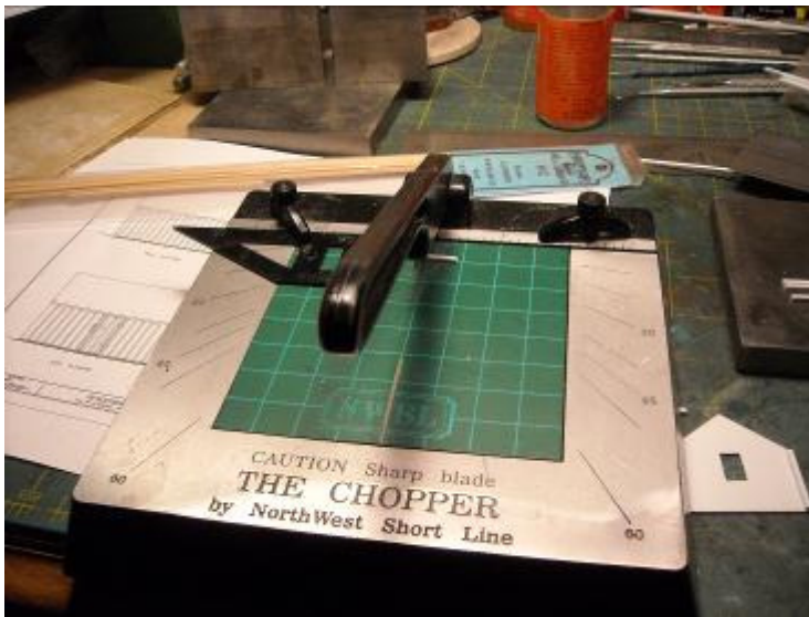
Photo #7 Using the North West Shorelines Chopper set to cut the supports.
